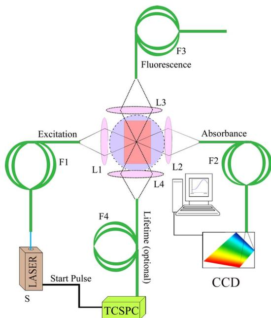
FIG. 1. (Color online) Schematic diagram of the universal setup. S is the source, F1–F4 are the optical fibers, L1–L4 are the fiber coupler lenses, and the violate circle represents the ambient light around the sample (reddish rectangle). CCD is the photosignal detector, connected with computer.
