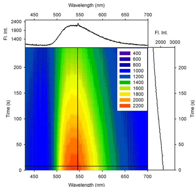
FIG. 4. (Color online) Wavelength (nanometer) vs time (second) contour plot of riboflavin in presence of UV-light. The above panel of the contour diagram is the full emission spectrum at time  $\sim 10$  s. The right hand side of the contour is the time dependent decay spectrum at  $\sim 540$  nm.
