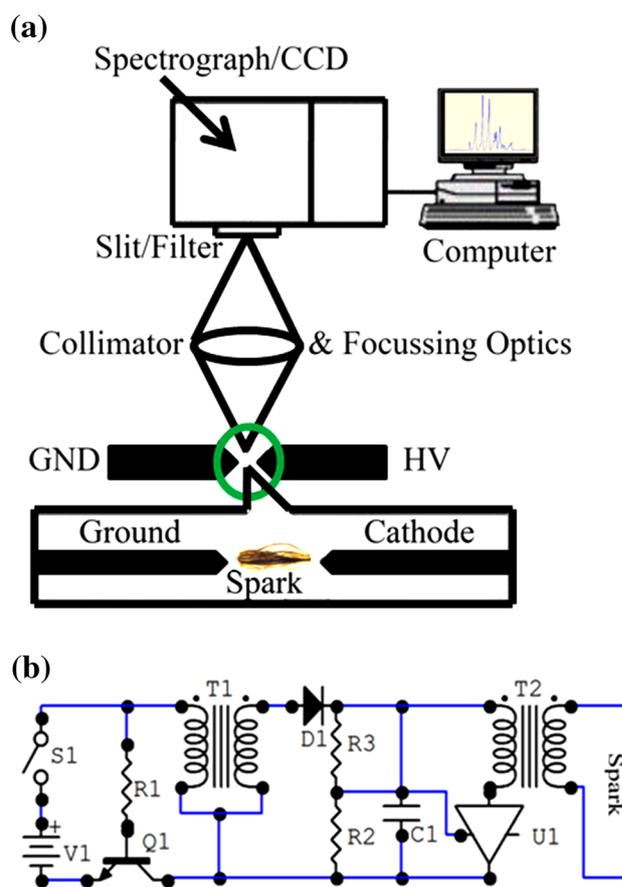
**Fig. 1** a Schematic diagram of the designed setup. b Circuit diagram of the battery operated high voltage power supply
