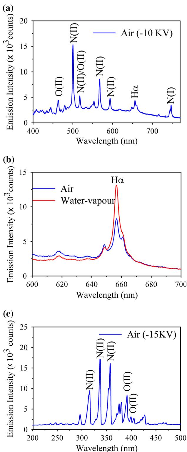
**Fig. 4** Benchmark spectra of air and water vapor from the designed setup
