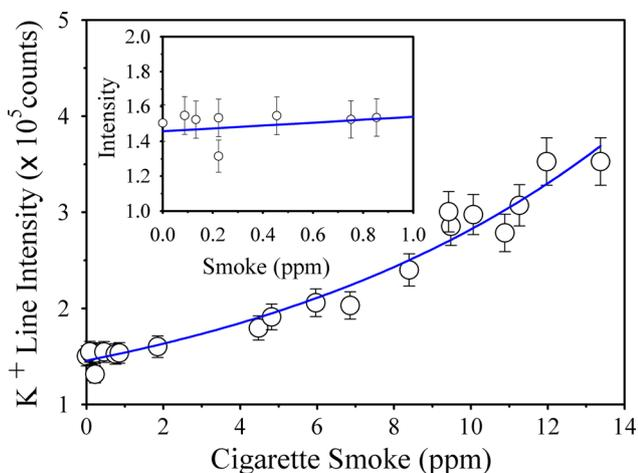
**Fig. 7** Intensity of the K<sup>+</sup> emission line in the cigarette smoke as a function of the concentration of the smoke in the gas chamber (open circles). The solid line is the guide to the eyes. Inset highlights low smoke concentration region, and the corresponding K<sup>+</sup> emission intensity revealing the sensitivity of our designed instrument
