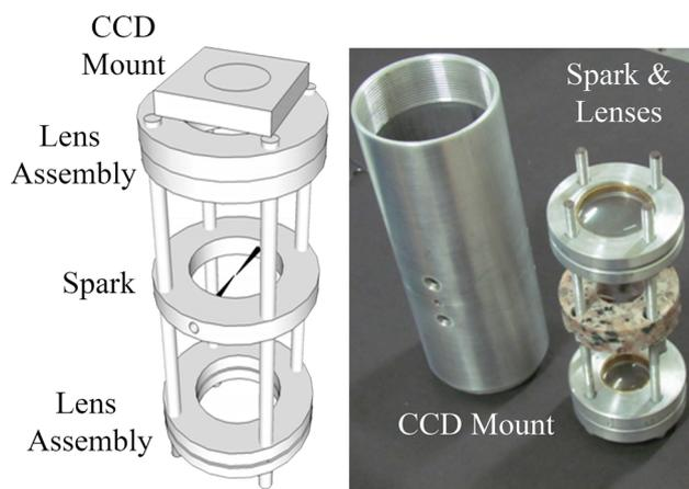
**Fig. 2** Mechanical design of the setup is shown in the *left panel*. *Right panel* shows photograph of the setup. Simplicity and portability can easily be evident from the picture
