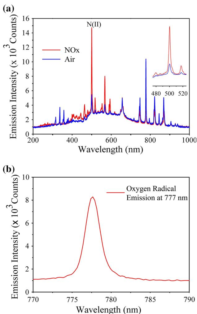
**Fig. 8** Detection of toxic  $\text{NO}_x$  (a) and highly reactive oxygen radical (b), using our setup
