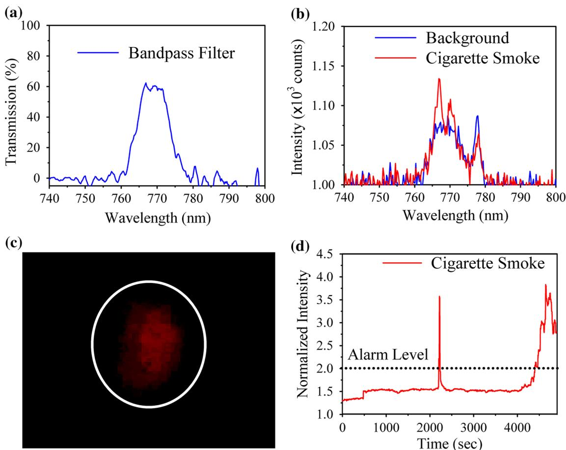
**Fig. 6** **a** Transmission characteristics of the optical filter used as a replacement of the costly spectrograph. **b** Spectrum of the cigarette smoke through the filter. **c** Signal acquired by computer through the
