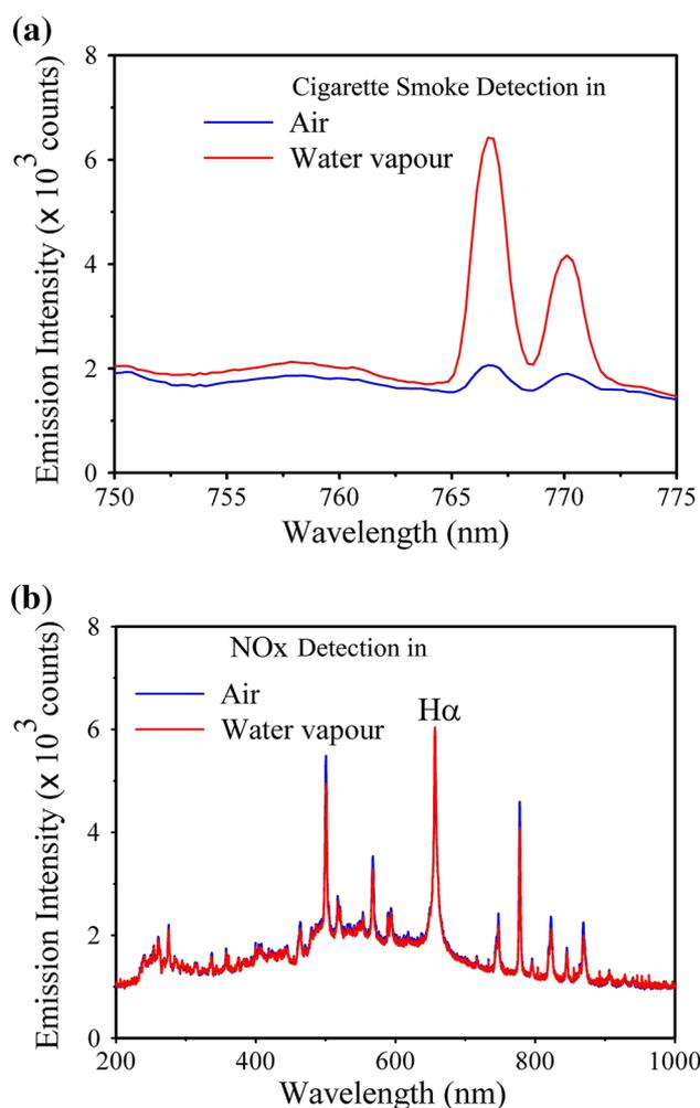
**Fig. 9** Detection of cigarette smoke (a) and  $\text{NO}_2$  in presence of water vapor (b). Enhancement of detection sensitivity in the case of cigarette smoke is clearly evident from panel
