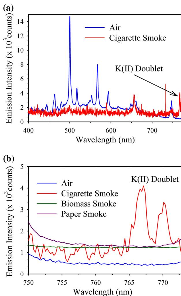
**Fig. 5** Spectroscopic detection of  $K^+$  ion emission as a distinct marker of cigarette smoke cow manure was used as a source of the smoke from biomass
