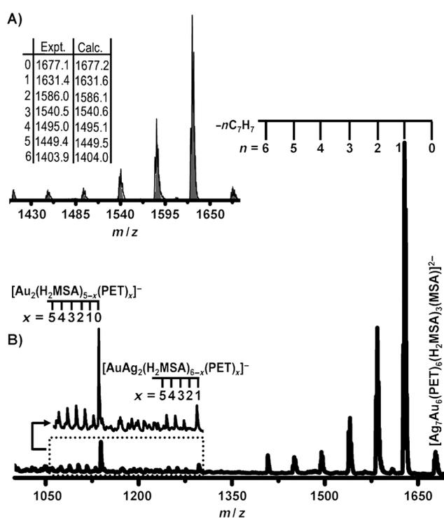
**Figure 3.** ESI MS spectrum of the PET-exchanged cluster in the negative-ion mode and in the region  $m/z$  1000–1700. Sequential loss of tropylium ( $n=0, 1, 2, \dots, 6$ ) was seen in ionization. The clusters show substitution of six ligands. The calculated isotope pattern is shown as gray under the experimental peak envelope in inset A. Inset B shows fragments.
