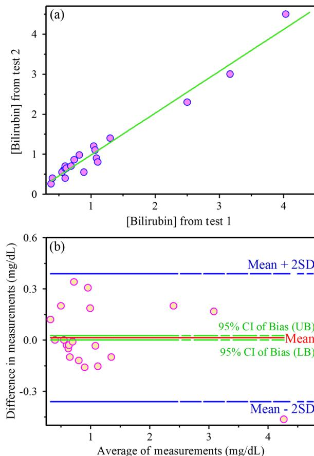
**Fig. 5** Stage II, reproducibility: (a) the linear regression plot of the TSB level measured successively by two different observers and (b) Bland-Altman analysis: reproducibility in measuring the TSB level by the device (see text).
