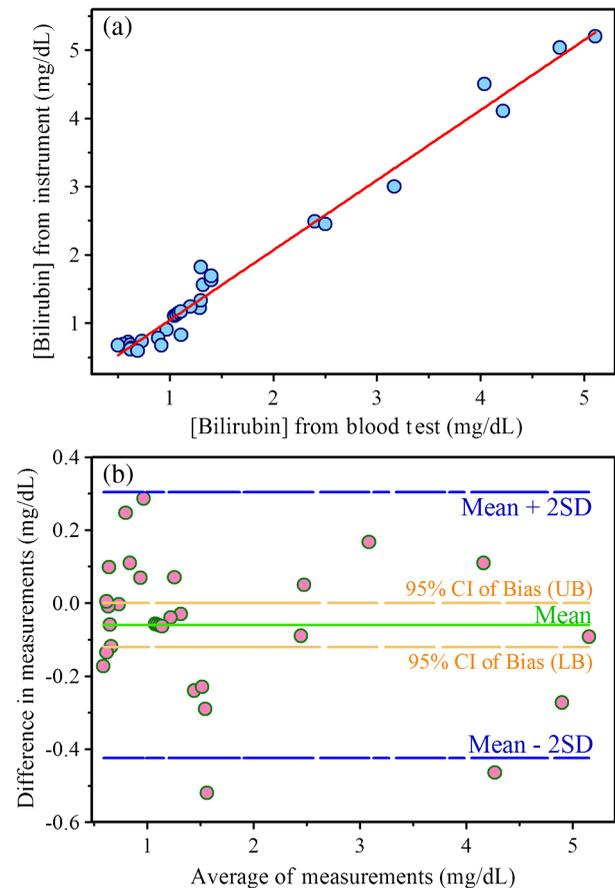
**Fig. 4** Stage II, statistical significance: (a) the linear regression plot of the TSB level measured in both the ways and (b) Bland-Altman analysis: difference against mean for the TSB data (see text).
